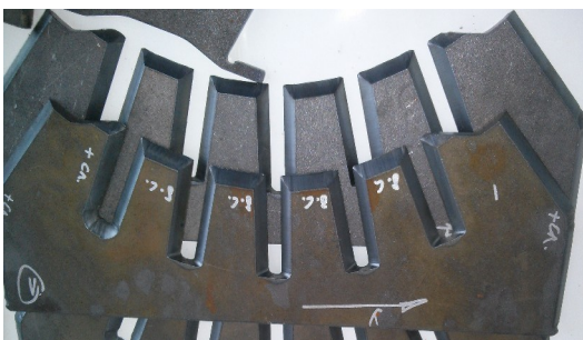
Fig.4: Part with complex bevels: project(up) and test parts(down)
